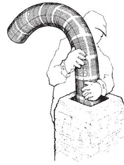
*It is easiest to pass the liner down from the top of the chimney. Position a helper inside at the fireplace or thimble to help guide the liner into final position.*
