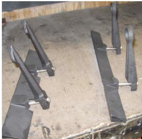
2. Spray a lubricant or penetrating oil on both of the bolts that attach the glass retainer and andiron to the backside of the front casting (WD-40, Break-Free CLP, Kroil, PB Blaster, etc). Let it work on the bolts up to 24 hours. Re-apply as necessary. Direct the spray under the retainer where the bolt passes through to the front frame.
