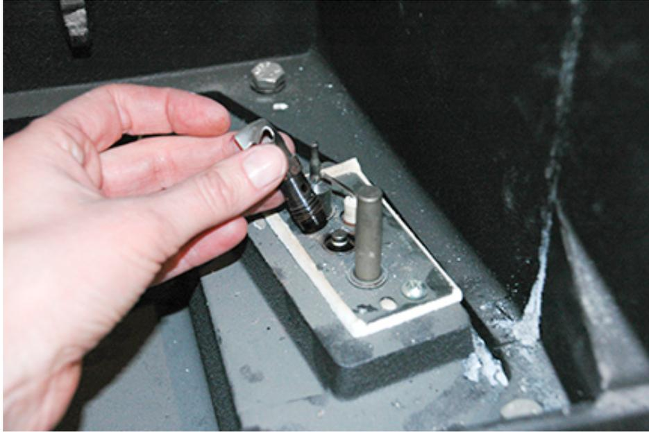
11. With the pilot removed, you will see the pilot orifice below. With your fingers or a pair of tweezers/pliers lift the pilot orifice out from the pilot assembly.
