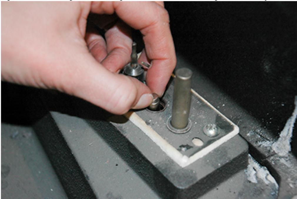
12. With the orifice out, you can inspect the orifice for clogging and clean with compressed air, alcohol, and/or a very thin gauge wire (be careful not to use a wire or pin larger than the orifice, you do not want to accidentally increase the orifice size).
