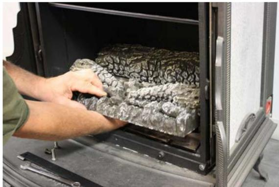
6. Lift the burner out of the firebox. Lift the front edge first then pull it up and out of the firebox. Natural gas stoves will have a narrow air shield attached to the burner.
