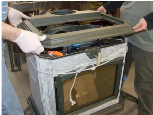
6. Remove the stone and replace it with the new one.
