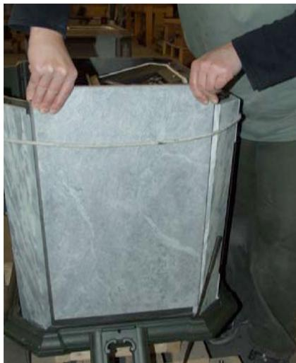
7. Carefully place the top frame back on the stove. As you lower the top down be careful not to break the edges of the stone by hitting them with the protruding buses where the tie rod is inserted on the bottom side of the top frame. Adjust the position of the stone as needed to avoid this damage.
